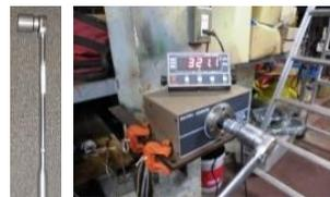
We calibrate the special torque wrench to 300 N · m using a digital analyzer before shipment.
