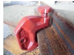
Be sure to put a mark on the bolt on one side.
