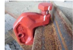
If you find the marks out of alignment, re-tighten the bolt with the special torque wrench.
